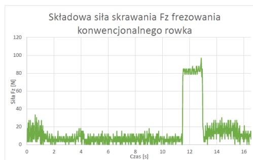
Fig. 5. Graph of the measured force component F_z during slot milling using the conventional method
