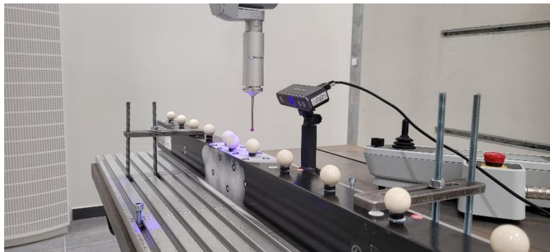
Fig. 3. Measurements of the reference object consisting of three spheres with both systems within the HMS
