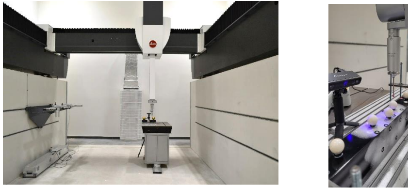
Fig. 1. Hybrid measuring system based on the use of an accurate large-volume coordinate measuring machine PMM-G 50.30.20 and a structured light scanner 3D Scanner MINI
