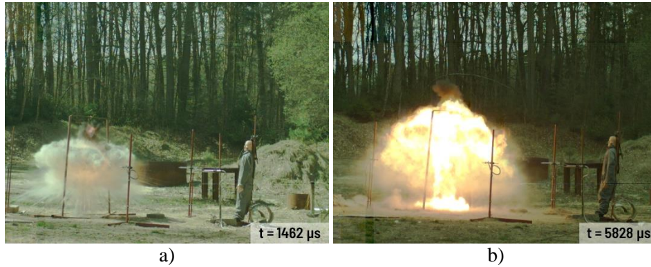
Fig. 1. Explosion of the tested charges: a) Amonal, b) Heksoflen
