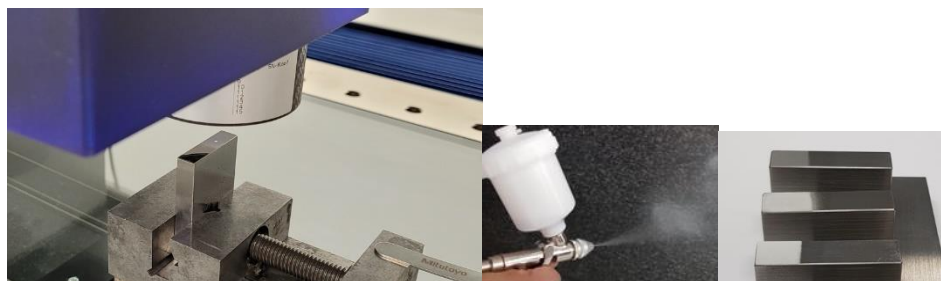
Fig. 1. Non-contact measurement with a white light sensor, Airbrush and matted gauge blocks
