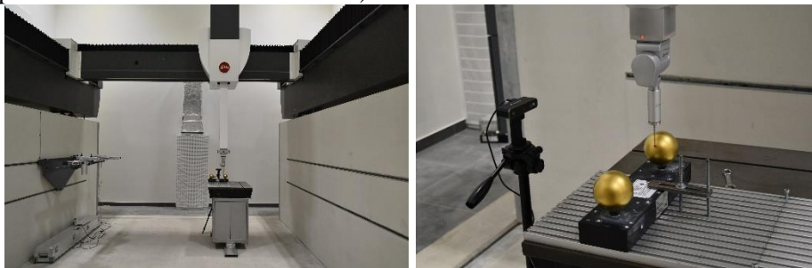
Fig. 4. Measurements of the standard sphere during tests no. I and II
