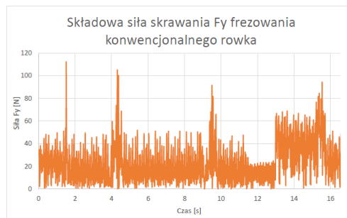
Fig. 4. Graph of the measured force component F_y during slot milling using the conventional method
