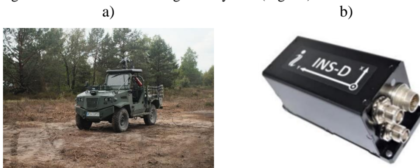
Fig. 1. View of developed TAERO vehicle (a) and installed GNSS INS module (b)
