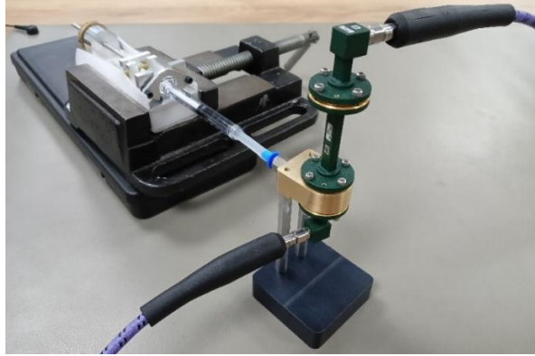
Fig. 2. A semi-open rectangular waveguide fixture for liquid permittivity measurements in WR22 standard (Q-band, 33-50 GHz) with a liquid dosing appliance
